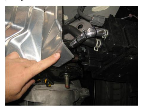
**4)** Now that the Evap cover is removed you need to wrap this fuel line with the heat wrap provided with your new exhaust system.
