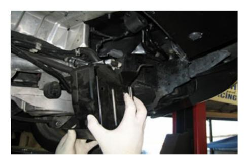
**3)** Bend the corner of the heat shield back to provide clearance for the passenger side muffler.
