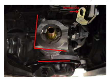
**17)** On the oil cooler assembly, remove the two dust covers from the top. Put a thin film of oil on the O-ring that is around the 2, Setrab supplied 8 AN fittings. This will ensure that, as you tighten the fittings in place, the O-ring does not bind on either surface and creates a good seal. You may now install and tighten down the 2, Setrab supplied 8 AN fittings. The wrench size is 1-1/16".
