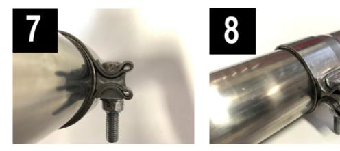
**13)** (Both Mufflers) Install FI-supplied 1/2" shaft collars on muffler hanger. Proper installation of shaft collar will be mated flush to the **forward vehicle side** of the OEM black rubber hanger.
