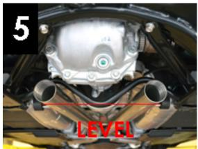
**7)** Reinstall the center cross brace. Use the supplied (4) shims washers, and (4) M8x 30mm flange bolts. When installed properly, the bottom of the x pipe should have clearance between the cross brace. The shim washers properly installed, go between the cross brace and the underside of the vehicle.
