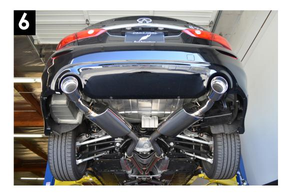
**12)** Verify that all 4 Accuseal clamps are as tight as image 7 shows and are in the proper location on the edge of the outer tubing with the slip fit, as shown in image 8. If your clamps do not mimic images 7 & 8, loosen them and adjust to match.
