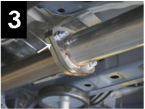
**NOTE:** Install 1 Accuseal clamp over the back of each lead tube before proceeding to the next step.
