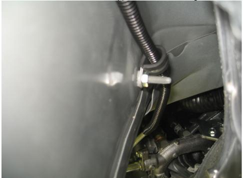
**23)** Repeat the identical process for the passenger side O2 sensor as step 22 with one exception. There is no clamp to tie the O2 sensor up in the passenger side of the transmission tunnel. Instead use the last zip tie we provided to secure it up to the transmission wiring harness as shown in the picture below.
