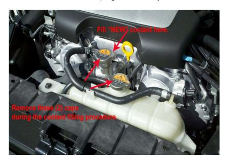
**C)** Reinstall both caps as shown in the picture above. On the inside of the white overflow tank you will see a MIN and MAX line. The coolant may seem high however, as soon as you start your vehicle, and the thermostat opens, the engine will take what it needs.
