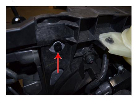
**B)** Add new coolant at the filler neck, as shown in the picture below. Using a funnel, fill up at a slow and steady pace until you see coolant begin to come out of the air relief hole at the top of the radiator. As soon as you see coolant coming out, reinstall the air relief plug immediately.
